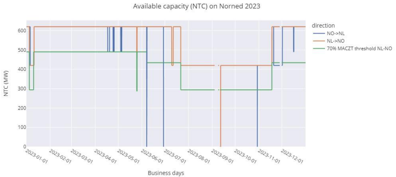
Figure 15: Available capacity (NTC) on the NL-NO2 bidding zone border. The values as included in the figure are including a correction for the application of implicit loss handling. Outages are filtered out of the dataset.
